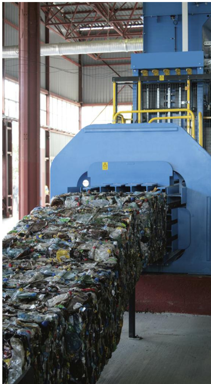
Bales of recycling exit a compactor
